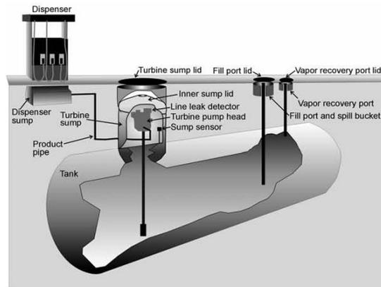
There are several types of sensors that are approved for UDC monitoring. The two common types are electronic and mechanical. Although they may function differently, both will stop flow of product at the dispenser when a leak is detected.
