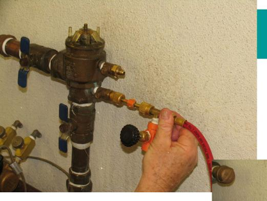
Connect the gauge to the bleed T on No. 1 test cock then open the No. 1 test cock to pressurize the gauge.
