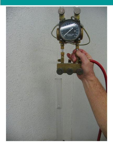
But holding it higher than the water in the column actually lowers the pressure causing this device to appear in failure.
