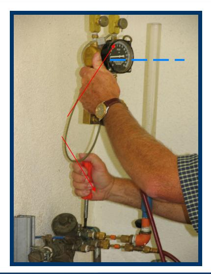
Close No. 2 and No. 3 test cocks, open Shutoff Valve #1 and move your test setup over so that the sight tube is on No. 4 test cock and the high side hose and compensation bleed T are on No. 3 test cock.
